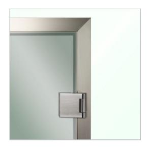
The GTWZ door frame is identical in appearance to the GTW clamping profile. GTW frames are pre-assembled and are supplied as two door jambs for the right-hand and left-hand sides plus a lintel. You carry out assembly on-site by simply screwing together the two inner brackets that are designed to connect the lintel and the jambs.
